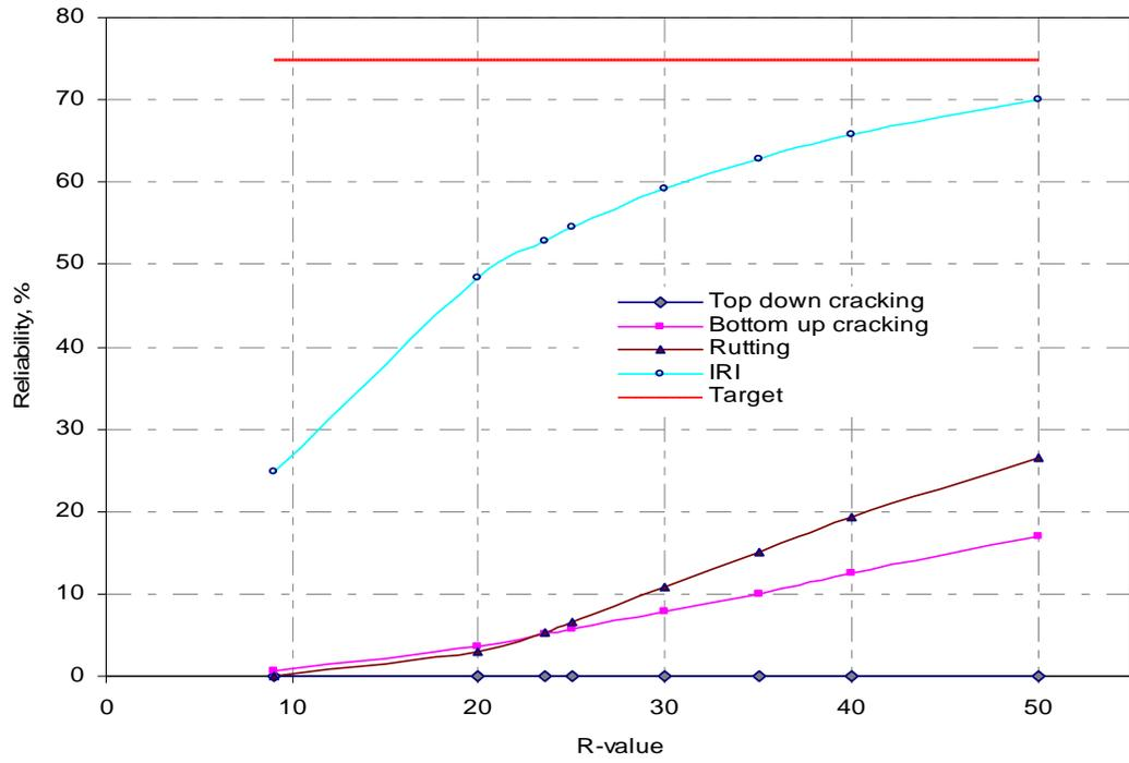
Figure 4.9 Evaluation of minimum *R-value* with MEPDG reliability output for NM 3
