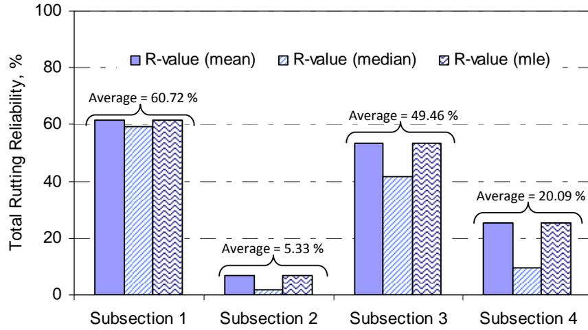
Figure 4.6 Comparison of total rutting reliability between sub-sections (US 54)
