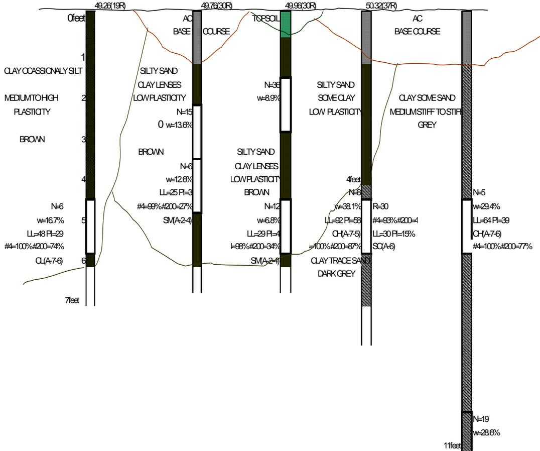
Figure 3.2 Typical soil profile of section 1
