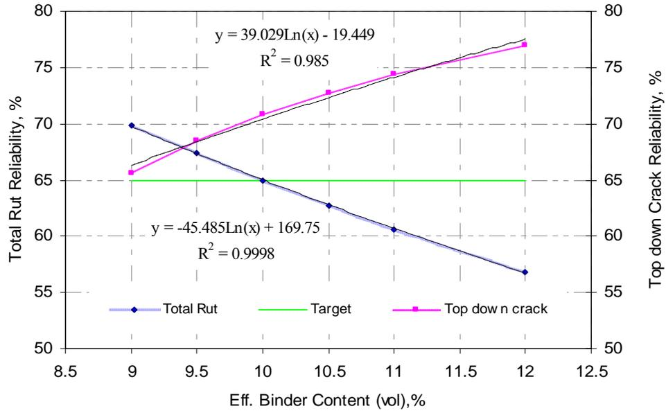
Figure 5.7 Effect of volumetric effective binder content on total rutting and top-down cracking reliability (NM 460/ NM 404)
