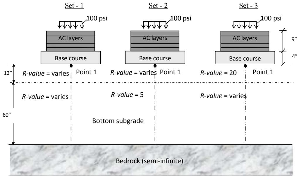
Figure 3.7 Pavement loading and section profile for linear elastic analysis
