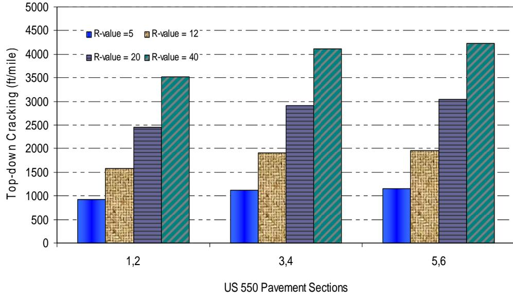
Figure 3.6 Effect of *R-value* on top down cracking
